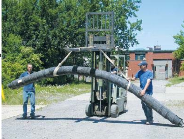
Photo submitted Workers transport a Tire Log via forklift. Re-Tread Products of Great Valley has been making Tire Logs, which are made of recycled tires, to use for a variety of demonstrations over the past five years.
